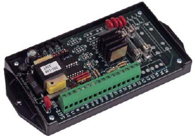
Typical applications include interfaces between utility metering devices and customer-owned energy control systems, demand recorder applications, or supervisory control systems (SCADA) interfaces. The RPR-22PS is particularly useful in applications where one channel is Kwh pulses and the second channel is Kvarh pulses.
