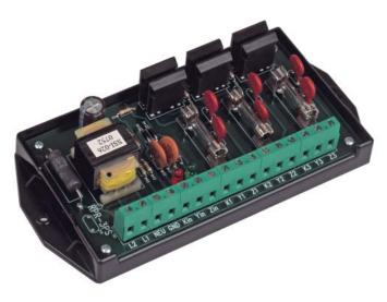
The RPR-3PS relay is designed to filter noise and transients from its input to prevent any false pulses at its output. Bright red and green LED indicators display the system's status at all times thus allowing a rapid visual check of the system's performance without requiring any additional test equipment.
