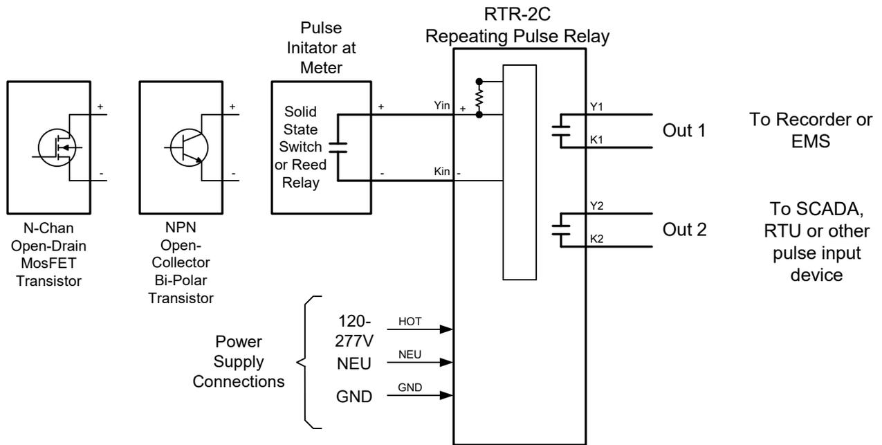
RTR-2C Repeating Pulse Relay Wiring Diagram
