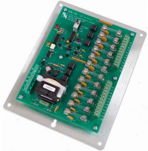
The SPR-112 relay has a switch-selectable input which can select the external Form A pulse input, the 1 Hz pulse generator or the internal variable pulse generator. Input filtering circuitry prevents noise from triggering the output. Pulses less than 18 mS are considered to be noise and will not be validated as a pulse. Once an input pulse greater in length than 18 mS is validated, the output will be changed to the state of the input.
