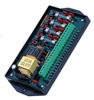
to the "K1in" and "K2in" terminals, the common return for both meters. Each output relay is switch-selectable to follow (echo) one of the two inputs, thus allowing each input to control one, two, three or even four relays. Flexible configurations for the two input channels are possible: 0/4, 1/3, 2/2, 3/1, and 4/0 such that one SPR-24 may be used in lieu of two or more relays to accomplish the same task.
