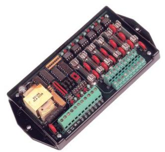
to each meter's Y and Z terminals from the SPR-36's Yin and Zin input terminals, returning to the Kin terminal, the common return for all meters. Since all meters supplying pulses to the SPR-36 have a common reference, a number of flexible input configurations can be wired.
