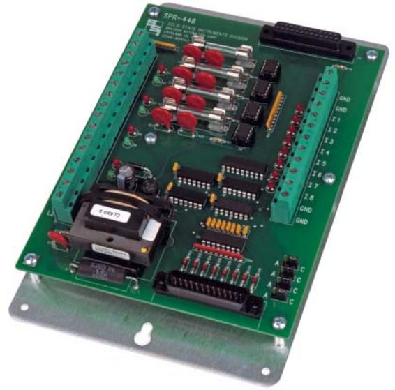
The input configuration of each input can be independently set on site as either a Form C (3-wire) or Form A (2-wire) input. The meter's pulse output "J3" wire harness plugs directly into the DB-25 connector, allowing for quick and convenient connection. Screw terminals are provided for each output making field wiring a snap.
