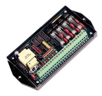
terminal, the common return for all meters. Since all meters supplying pulses to the SPR-44 have a common reference, a number of flexible input configurations can be wired. For example, two inputs can be wired in parallel giving a "splitting" configuration where one input and two outputs is desired.
