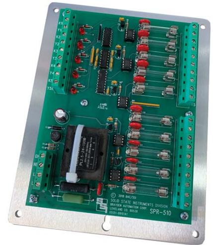
The SPR-510 relay's Form A inputs feature input filtering circuitry to prevent noise from false triggering the outputs. Pulses less than 18 mS are considered to be noise and will not be detected as a valid pulse. Once an input pulse, greater in length than 18 mS, is detected the corresponding outputs will be changed to match the state of the input.
