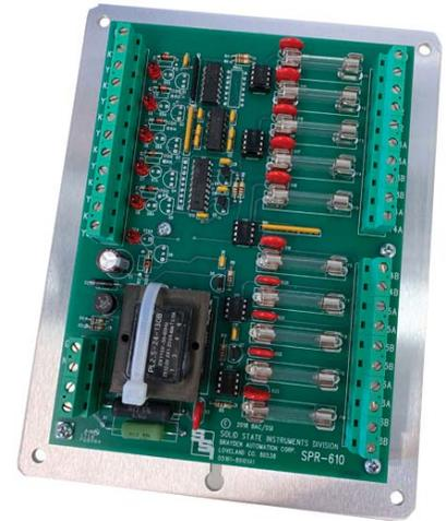
The SPR-610 relay's Form A inputs feature input filtering circuitry to prevent noise from false triggering the outputs. Pulses less than 18 mS are considered to be noise and will not be detected as a valid pulse. Once an input pulse, greater in length than 18 mS, is detected the corresponding outputs will be changed to match the state of the input.
