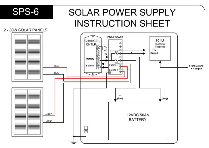
**MOUNTING POSITION** - The SPS-6 Enclosure must be mounted in an upright position so that the battery is placed on the <u>bottom</u> of the enclosure. Mount the solar panels using the metal mounting systems provided to get the correct mounting angle pursuant to the instructions included in the mounting bracket kits. The solar panel mounting bracket is designed to attach to a pole or building. Solar Panels may not be shaded by trees or a building at any time.
