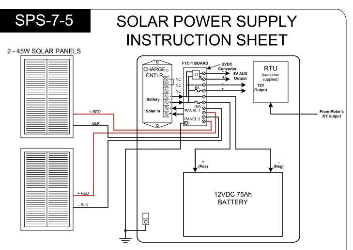
**<u>MOUNTING POSITION</u>** - The SPS-7-5 Enclosure must be mounted in an upright position so that the battery is placed on the <u>bottom</u> of the enclosure. Mount the solar panels using the metal mounting systems provided to get the correct mounting angle pursuant to the instructions included in the mounting bracket kits. The solar panel mounting bracket is designed to attach to a pole or building. Solar Panels may not be shaded by trees or a building at any time.
