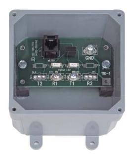
modem from lightning or other electrical disturbances that may affect the telephone line inside the home or business. A number of mounting options are available (listed below) and a gasketed lid ensures that the circuit inside remains dry and clean.
