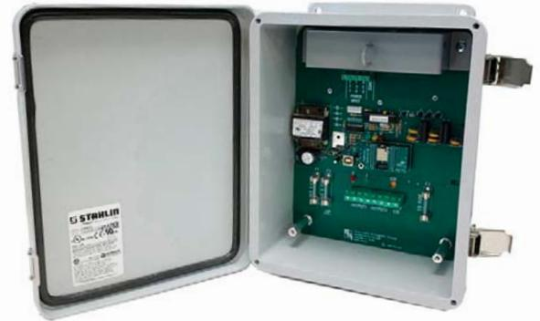
The WPG-1SC features integral Wifi radio module and two KYZ pulse outputs, in a polycarbonate NEMA 4X enclosure. As the WPG-1SC receives periodic data from utility's meter, the data is read and interpreted to obtain the current demand information. Accumulated energy is computed, and pulses are outputted according to a selected pulse value.
