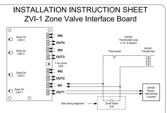
**PURPOSE** - The ZVI-1 is an interface between the 24VAC thermostat loop and an electromechanical counter that records usage. Usage is measured per second. Once 60 seconds have incremented, the counter receives a pulse signal to increment its count by 1. In this manner, the counter displays the number of minutes that its respective Zone Valve has been on.
