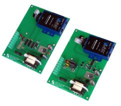
received by the EPR-1 the pulse information is decoded, validated and implemented into the correct pulse output state. The output is configured as a Form C, but can be used as either a Form A (2-wire) or a Form C (3-wire) depending on the transmitter's input configuration selection. The EPR-1 receiver requires an EPT-1 transmitter to create the EPL-1 ethernet pulse link system. Both the EPT-1 and EPR-1 require a static IP address so that they can communicate with each other.
