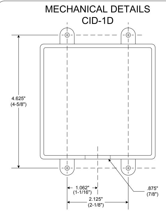
Enclosure has one pre-drilled 7/8" hole for 1/2" conduit connections.
