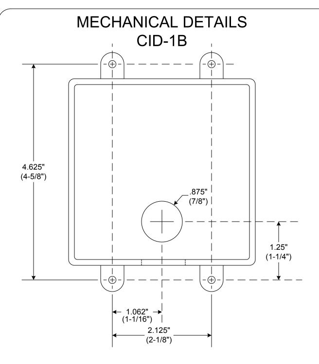
Enclosure has two pre-drilled 7/8" holes for 1/2" conduit connections.
