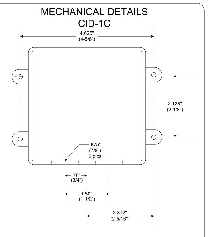
Enclosure has two pre-drilled 7/8" holes for 1/2" conduit connections.
