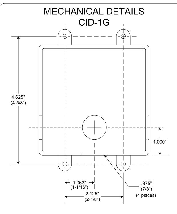
Enclosure has four pre-drilled 7/8" holes for 1/2" conduit connections.
