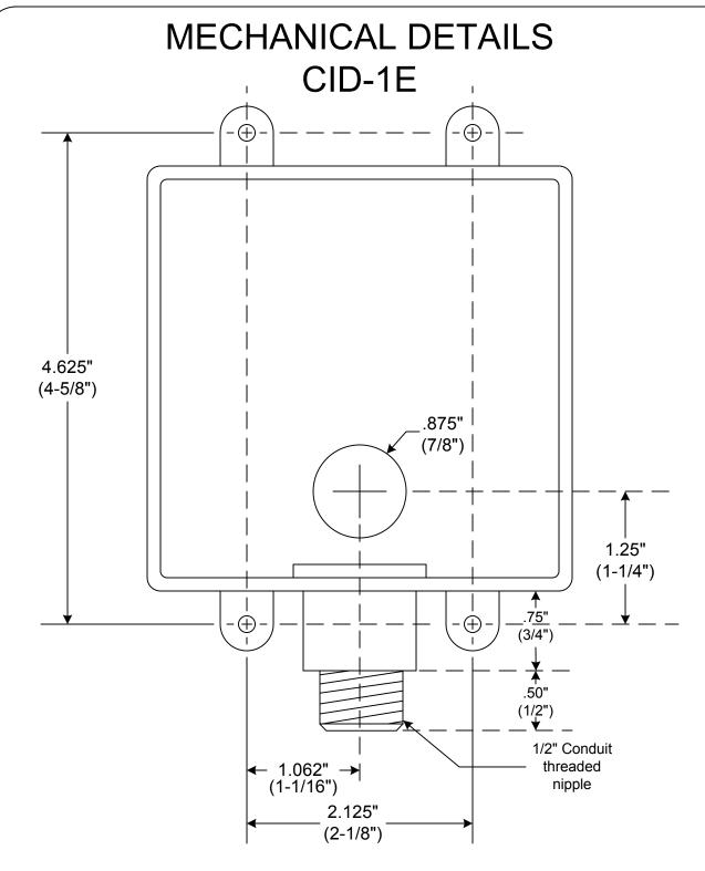
Enclosure has one 1/2" threaded nipple for connection to electrical enclosure.
