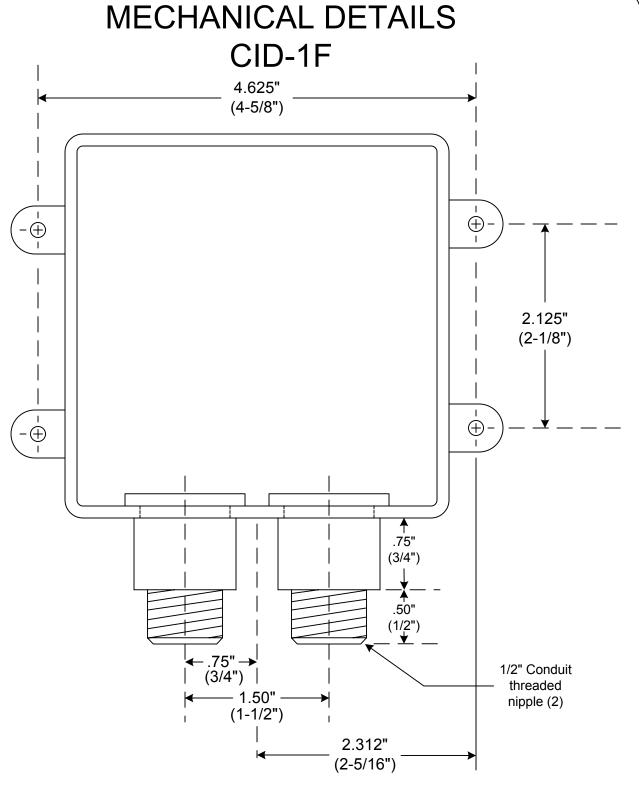
Enclosure has two 1/2" threaded nipples for connection to electrical enclosure.
