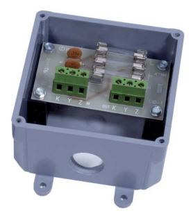
installed in the terminals "slot", no conductive parts are exposed on the surface of the terminal strip, thus allowing the user maximum protection from accidental electrical shock. Each lead of the CID-1 is individually fused to prevent damage to the meter or the customer's energy control system. In addition, a built-in "snubber" network is installed to suppress excessive transient voltages.
