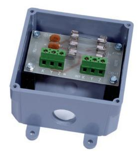
installed in the terminals "slot", no conductive parts are exposed on the surface of the terminal strip, thus allowing the user maximum protection from accidental electrical shock. Each lead of the CID-1 is individually fused to prevent damage to the meter or the customer's energy control system. In addition, a built-in "snubber" network is installed to suppress excessive transient voltages.
