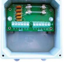
wire has been correctly installed in the terminals "slot", no conductive parts are exposed on the surface of the terminal strip, thus allowing the user maximum protection from accidental electrical shock. The "K" lead of each CID-2 channel is fused to prevent damage to the meter or the customer's energy control system. In addition, a built-in "snubber" network is installed to suppress transient voltages or other electrical noise related to contact opening.
