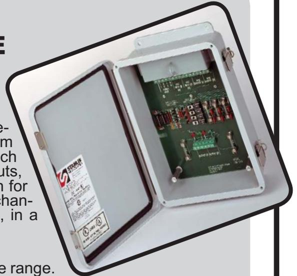
The CIR-24S dual repeating pulse isolation relay is designed to provide four isolated dry-contact, solid-state Form C (K, Y, & Z) outputs from two Form A or C inputs. Each output is mappable (assignable) to either of the two inputs, allowing a flexible configuration. The primary application for the CIR-24S is where two independent isolation relay channels are desired with multiple outputs on each channel, in a weather-tight package.
