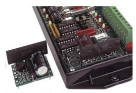
The DCS-1 uses a switching power supply technology that converts 125VDC to +12VDC without any heat being generated, thus eliminating any power dissipation problems usually associated with linear power supplies.
