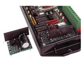
the DCS-1 supplies the relay's power supply requirements as well as providing a wetting voltage to the meter.
