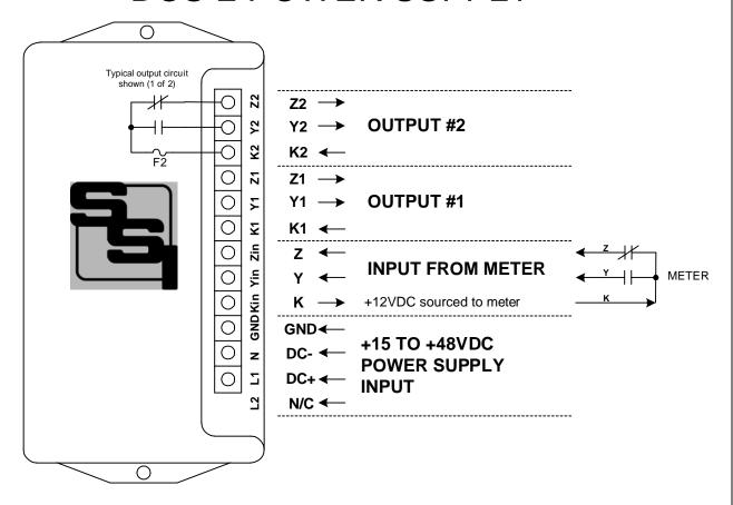
**SUMMARY** - This addendum accompanies any SSI Pulse Isolation Relay is equipped with the DCS-2 Power Supply option. This option allows you to power your relay from a DC voltage source over a range of +15 to +48VDC.
