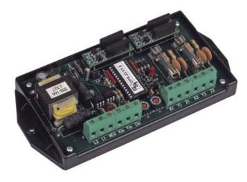
with a small screwdriver. The DPR-22 microcontroller checks the input pulses for the correct sequence and timing, and counts the input pulses for division only when a correct and valid sequence of pulses occur, thus assuring a high degree of noise rejection. Two sets of bright red and green LED lamps indicate the input and output status of the system at all times thus allowing a rapid visual check-out of the system's performance without requiring any additional test equipment.
