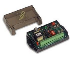
the input preset count is reached. In pulse mode, a 100mS output pulse is generated when the preset count is reached. Pulse count is stored in non-volatile EEPROM memory so that any power failure will not lose the current pulse count. In the event that the divider ratio is low and pulse rate is high in the pulse output mode, the microcontroller will store up to 255 output pulses waiting to be output. This output pulse number is also stored in EEPROM memory, so that no pulses are lost.
