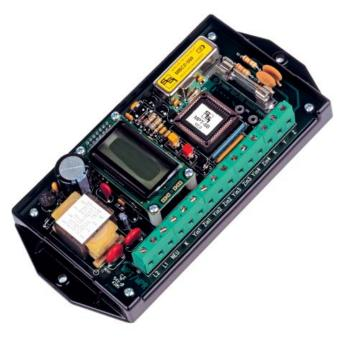
display at any time without disturbing the operation of the unit. Typical applications include interfaces between utility metering devices and customer-owned energy control systems, demand recorder applications, and supervisory control systems (SCADA) interfaces. The input pulse signal from the sending device to the MPR-4 is by four sets of "Y" & "Z" leads with a common "K" lead.
