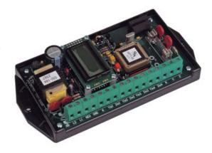
applications, and supervisory control systems (SCADA) interfaces. The MPT-4B pulse totalizer may also be used as a pulse value translator if it is desirable to translate odd pulse values such as 0.1234 KWH/pulse to an even value, 0.5000 KWH/pulse. The pulse inputs of the MPT-4B are configured as four sets of Y & Z input terminals with a common "K" input terminal.
