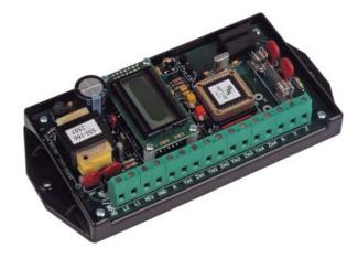
pulse totalizer's pulse inputs are configured as four sets of Y & Z input terminals with a common "K" input terminal.
