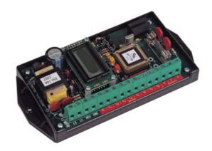
tions, and supervisory control systems (SCADA) interfaces. The MPT-8B pulse totalizer may also be used as a pulse value translator if it is desirable to translate odd pulse values such as 0.1234 KWH/pulse to an even value, 0.5000 KWH/pulse. The pulse inputs of the MPT-8B are configured as eight sets of Y input terminals with a common "K" input terminal.
