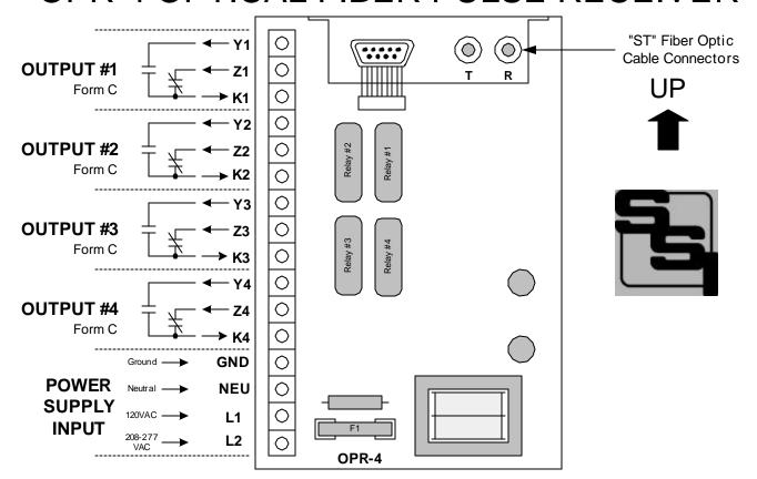
**MOUNTING POSITION -** The OPR-4 MUST be mounted in a vertical position, as shown above.
