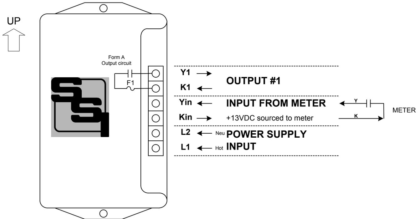
**MOUNTING POSITION** - Because the PIR-1 contains a mercury-wetted relay, it must be mounted in a vertical position to operate correctly.
