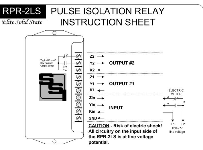
**MOUNTING POSITION** - The RPR-2LS can be mounted in any position.
